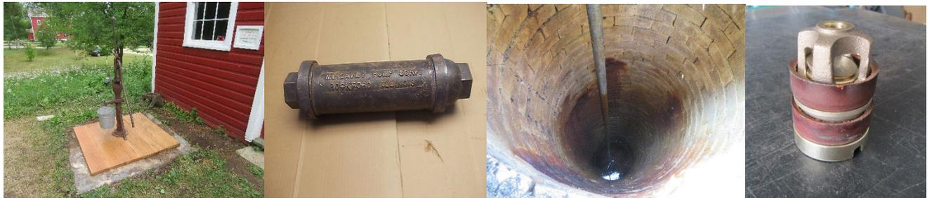
(From left to right) Our W. L. Davey pump / Pump cylinder attached to the pipe below the water level / 20’ deep well with 6’ of standing water and cream city brick lining / Mechanism which fits inside the cylinder and lifts the water with each stroke.
